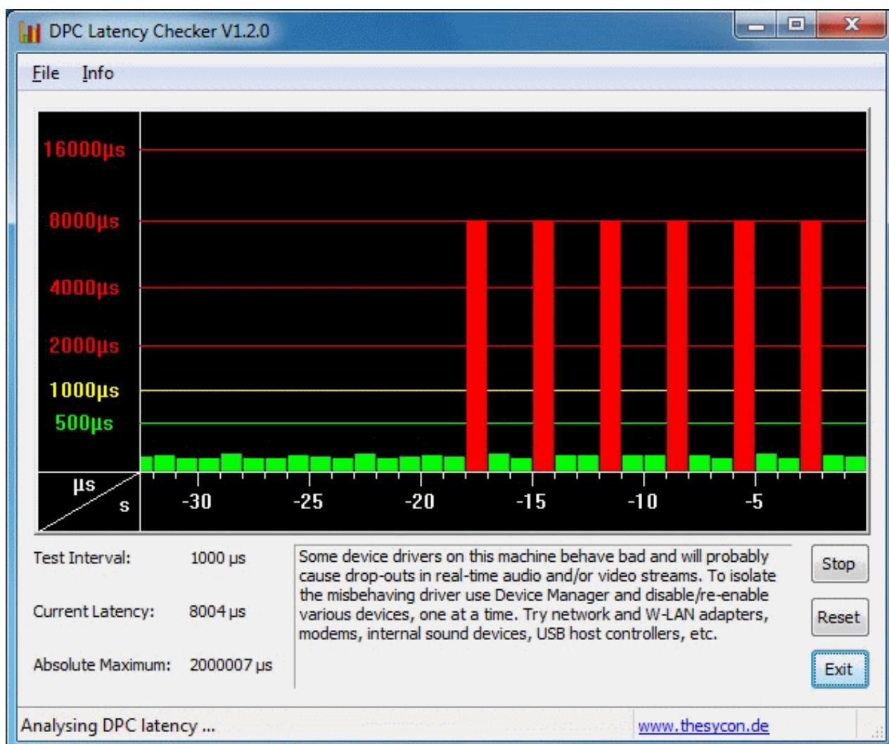
At a period of 3 seconds a kernel-mode driver in the system is stalling the CPU for about 3.5 milliseconds. So every 3 seconds DPC latency is exceptional large and drop-outs in real-time data streams will typically occur.
